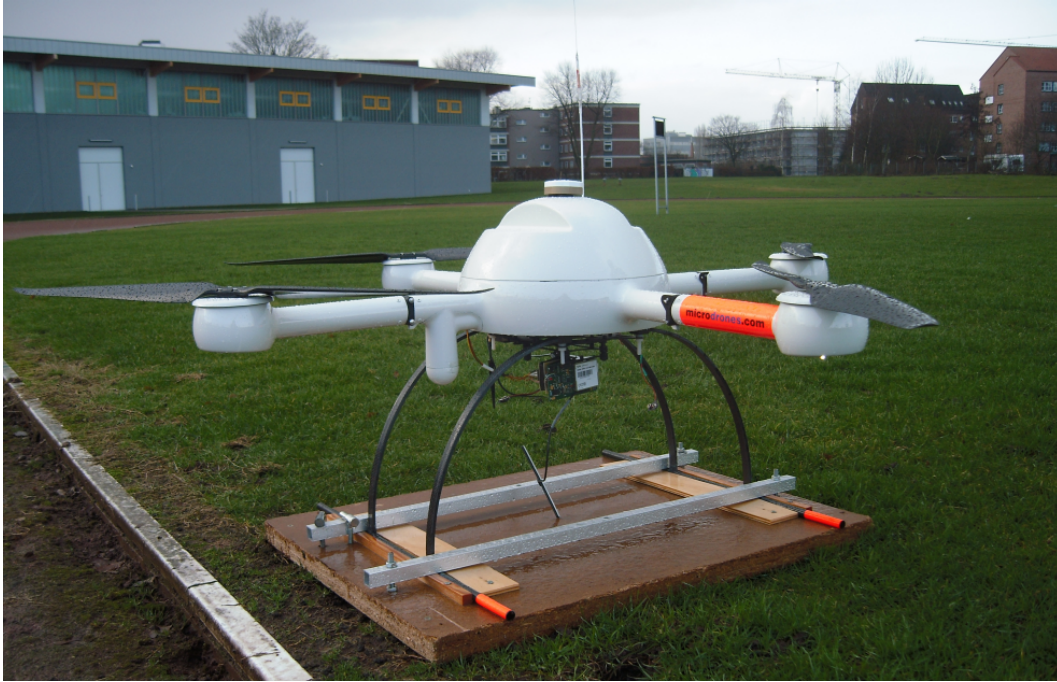
Figure 6.1.: Static position measurement of a MD4-1000 with mounted DGNSS-based positioning system on a predefined GCP.
